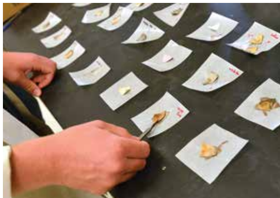
Water filter samples have silver deposited on their surfaces from various silver salt/tea bath combinations. – VMI Photo by John Robertson IV.
